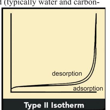
tity adsorbed at each pressure (and temperature) defines an adsorption isotherm, from which the quantity of gas required to form a monolayer over the external surface of the solid is determined. With the area covered by each adsorbed gas molecule known, the surface area can be calculated.
