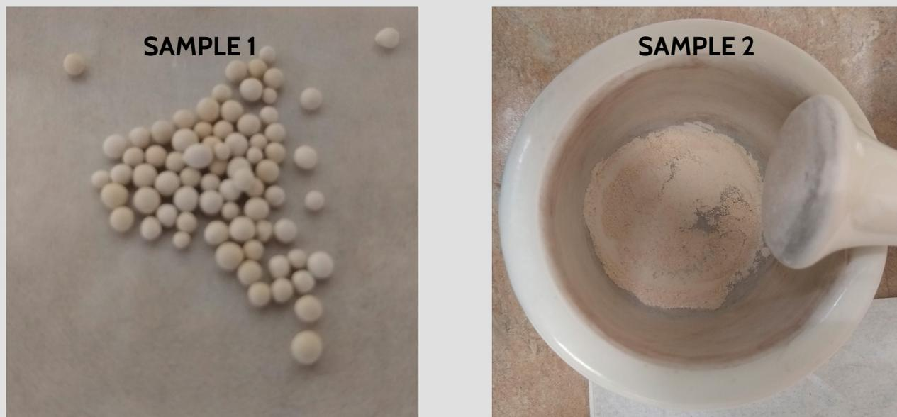
**Figure 3.** (left) Sample 1 – Pelletized Zeolite 13X (right) Sample 2 – Crushed Zeolite 13X
