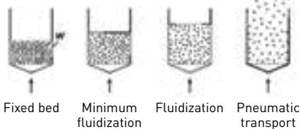
**Fluidized bed reactor** with differential pressure measurement.
