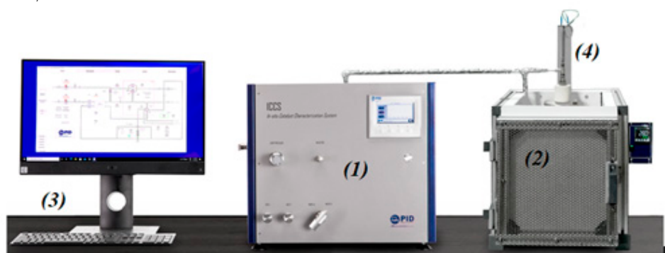
Figure 1. The ICCS commercial system connected to an external reactor placed in a programmable oven. (1) In Situ Catalyst Characterization System (ICCS). (2) Stand-alone programmable oven. (3) Computer to register and reduce data. (4) 9 mm SS316 tubular reactor.
