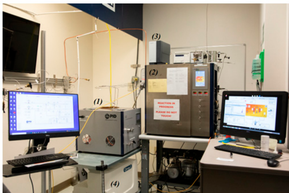
Figure 2. Shows equipment used in characterizing and testing catalysts for this work. (1) The In Situ Catalyst Characterization System (ICCS). (2) The FR-100 microreactor. (3) The micro-gas chromatograph. (4) The MKS mass spectrometer.
