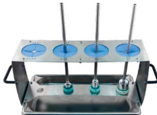
Penetrometer Rack: 15cc, 5cc, 3cc.
