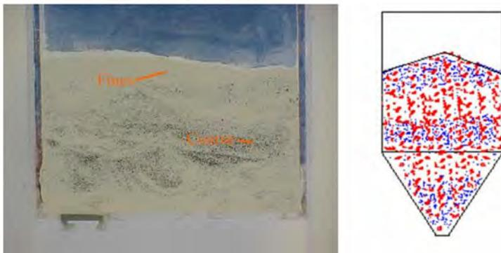
Fig 4. Typical impact fluidization segregation
