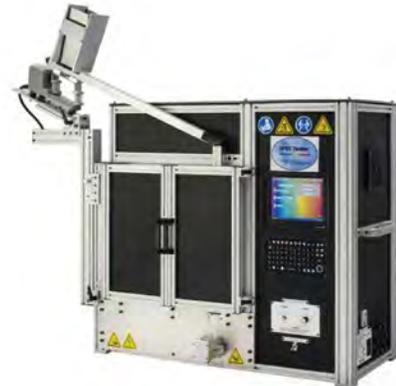
Figure 4. SPECTester used in Segregation Analysis
