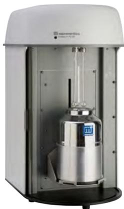
resulting in increased error. Normally for materials with low surface areas, the amount of material is maximized in order to increase this difference ( $V_i - V_e$ ). Unfortunately this approach has an upper limit depending on the size of the sample tube and the physical properties of the material. Another approach is to use an alternate analysis gas.
